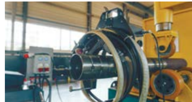
An MWG-170 open-type torch for welding Ø50÷168 mm pipes, with an MWA-400 Panasonic welding power supply
