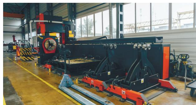
For pipe stock cutting and facing we employ a MEBA bandsaw machine and a COPIER beveling machine
